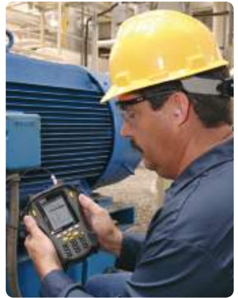
Recording vibration values using an SKF Microlog series data collector
